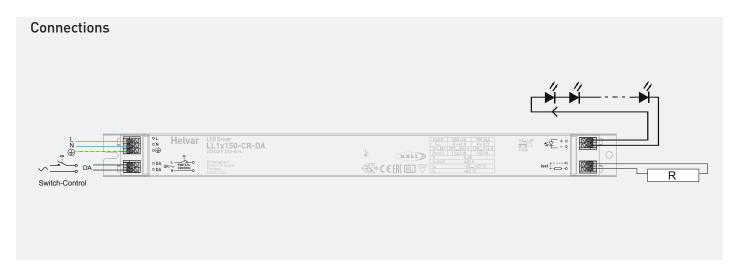
The resistor/current setting values are then adjusted according to the LEDset specification. The resistor value for each required output current can thus be calculated from the formula R ( $\Omega$ ) = (5 V) / I\_out \* 1000. In the table below are presented some resistor values across the whole current range.
